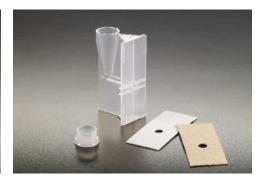
Fully compatible with the Shandon CytoSpin® Centrifuge, Simport CytoSep™ Cytology Funnels can be used to deposit a thin layer of cells in a clearly defined area of a microscope slide. The filter card absorbs any excess fluid. These Cytology Funnels have the filter cards pre-attached for consistent, reliable results. No alignment necessary! All disposable Funnels are packaged with closure caps to seal in specimen for added protection. All components also available separately.
