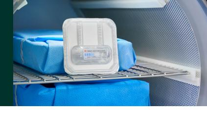
The first ever preassembled VH2O2 test pack contains both a CI and BI
